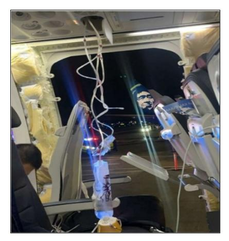
330. The following photo shows the size of the hole that resulted when the door plug flew out the side of the plane.
